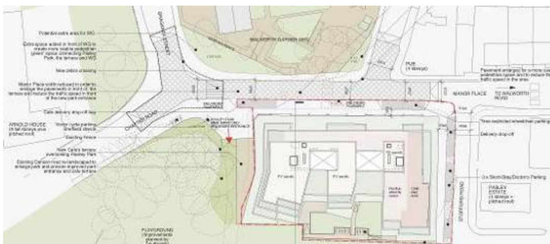
Proposed highway works around the application site
